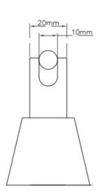
Materials: Constructed from stainless steel with exposed surfaces brushed or polished finish.
