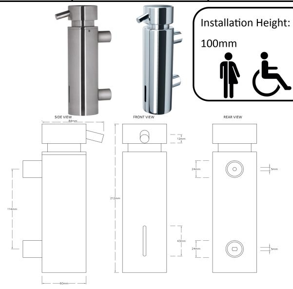
Materials: Constructed from chrome plated brass with exposed surfaces brushed or polished finish.
