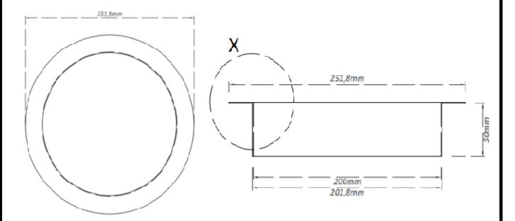
Materials: Constructed from Type UK 304 stainless steel, 0.9mm gauge with exposed surfaces in a brushed satin finish.
