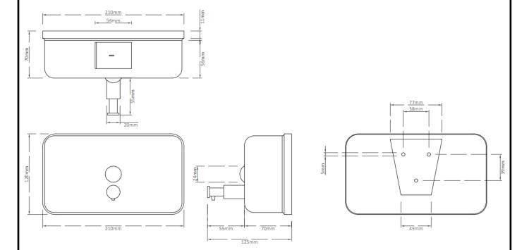
Materials: Constructed from type 304 stainless steel, exposed surfaces are in a brushed finish.
