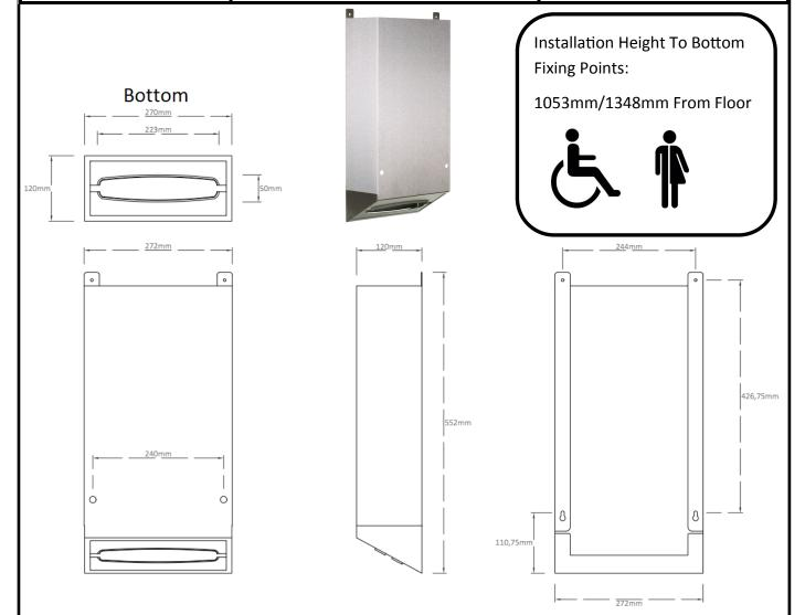
Materials: Constructed from high quality stainless steel, exposed surfaces brushed finish.
