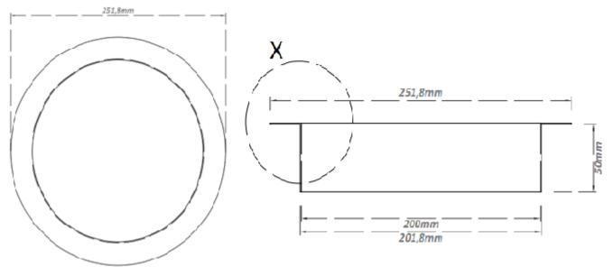
Materials: Constructed from Type UK 304 stainless steel, 0.9mm gauge with exposed surfaces in a Black Matt finish.
