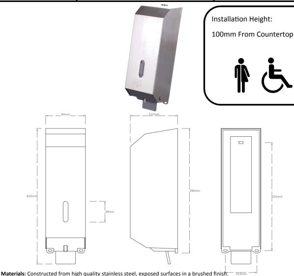
**Installation:** Unlock dispenser and remove filling reservoir. Mark a hole through the top central fixing indicator on the wall 360mm above the countertop and drill hole then insert plug, mark two further fixing points 255mm below, drill and insert plugs. Secure the unit to wall using screws provided. The soap dispenser will sit 100mm above countertop.
