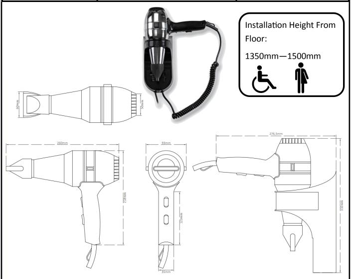
Materials: Constructed from stainless steel and ABS.
