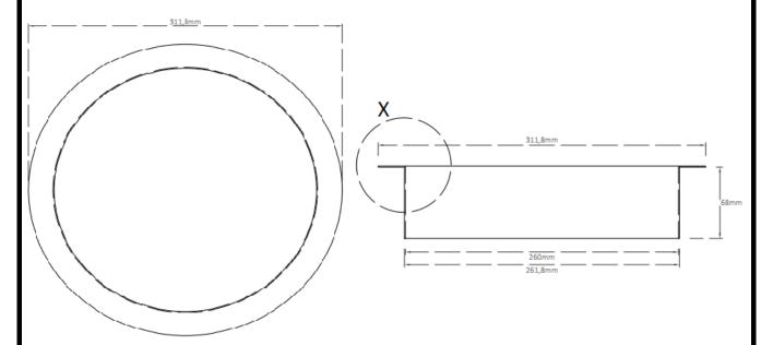
Materials: Constructed from Type UK 304 stainless steel, 0.9mm gauge with exposed surfaces in a brushed satin finish.
