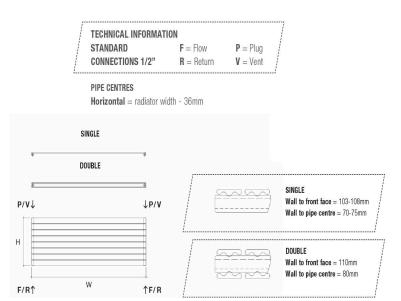
MaterialsSteelConnections½" Flow and ReturnTest Pressure6 BarTesting AuthorityEN442Max operation pressure4 BarMax working temperature90c
