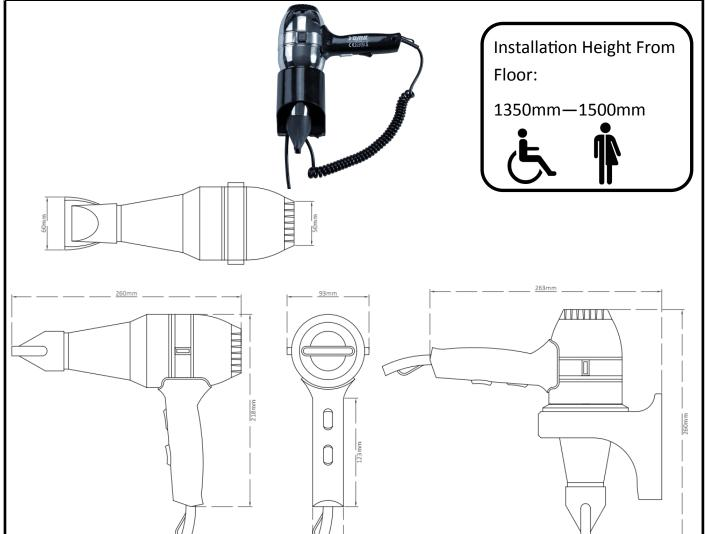
Materials: Constructed from stainless steel and ABS.
