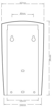
Materials: Constructed from type 304 stainless steel, exposed surfaces are polished finish.
