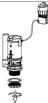
Remove the nut and nut collar from flush valve base.Don't remove the seal !!!
