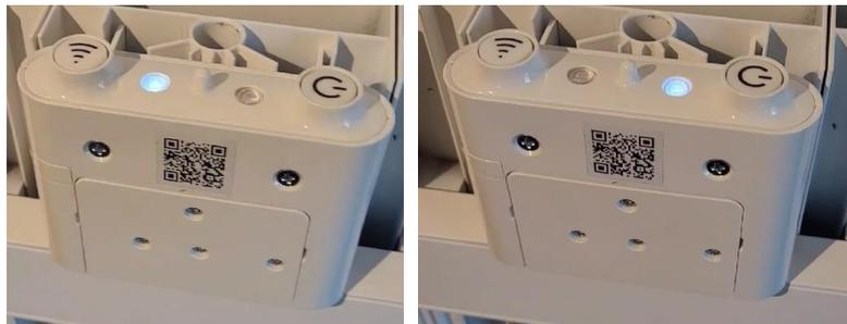
The unit will then beep 5 times followed by a further sequence of flashing lights. Then after approximately 30 seconds the unit will be a further 5 times and both lights will be steady. The unit will then beep 5 more times and a green light will display to indicate the reset is complete (see below).
