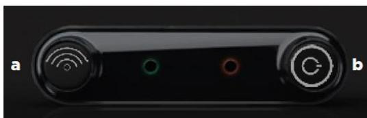
Press the WiFi button (a) on the thermostat control to enter pairing mode.
