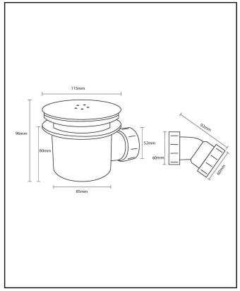
Dimensions (Measurements in mm)
