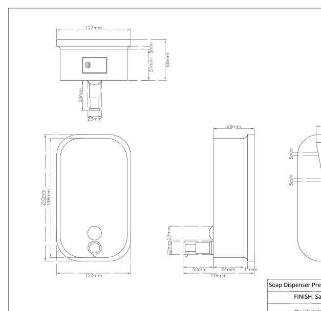
Weight when empty: 0.8kg Lockable and vandal resistant Compatible with liquid pearl soaps only Glass level indicator One shot action 1.2ml 1000ml capacity for heavy use
