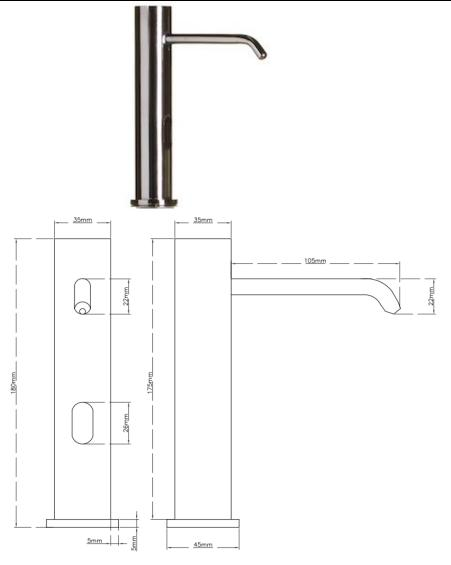
Materials: Constructed from Type UK 304 stainless steel, 0.9mm gauge with exposed surfaces in a polished finish.
