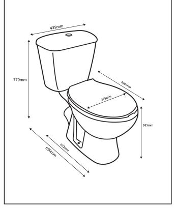
Dimensions (measurements in mm)
