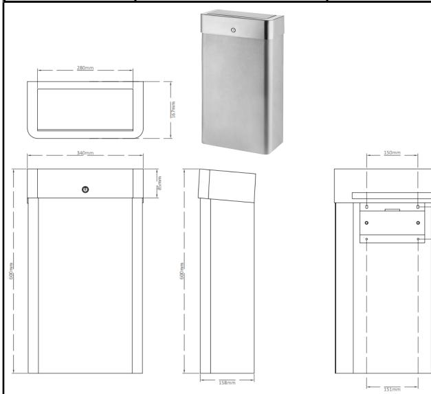
Materials: Constructed from type 304 stainless steel, exposed surfaces in a brushed finish.
