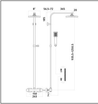
Dimensions (measurements in mm)
