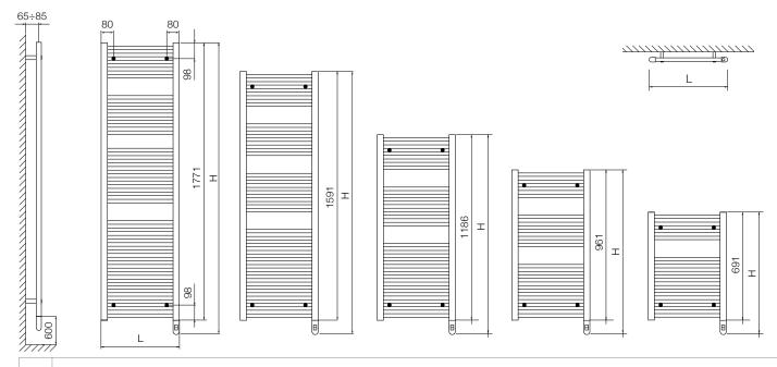
The exact order of the tubes and of the "openings" between the tubes themselves is that one showed in the technical drawings above; the picture in the page aside can sometimes be only apprroximate (regarding tubes and of the "openings" between the tubes themselves)
