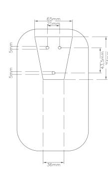
Materials: Constructed from type 304 stainless steel, exposed surfaces are in a brushed finish.
