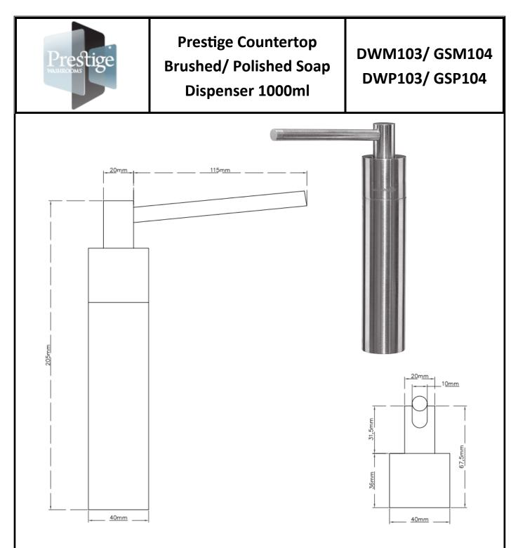
Materials: Constructed from stainless steel with exposed surfaces brushed or polished finish.
