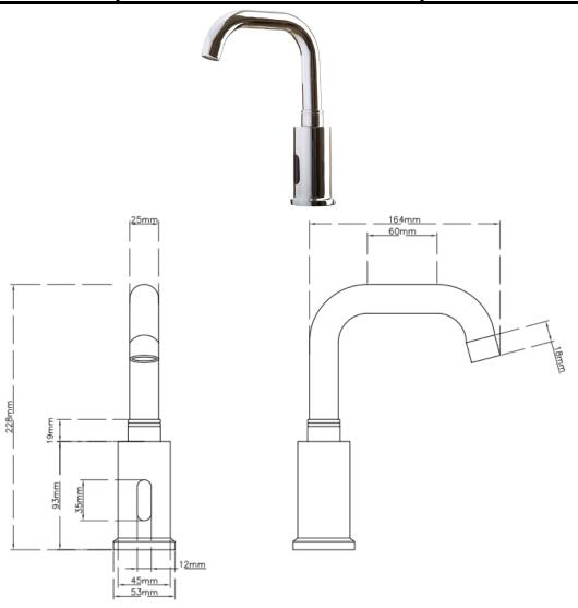
$\textbf{Materials:} \ \textbf{Constructed from chrome plated brass with exposed surfaces polished finish.}$
