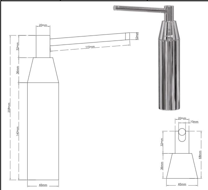
Materials: Constructed from stainless steel with exposed surfaces brushed or polished finish.
