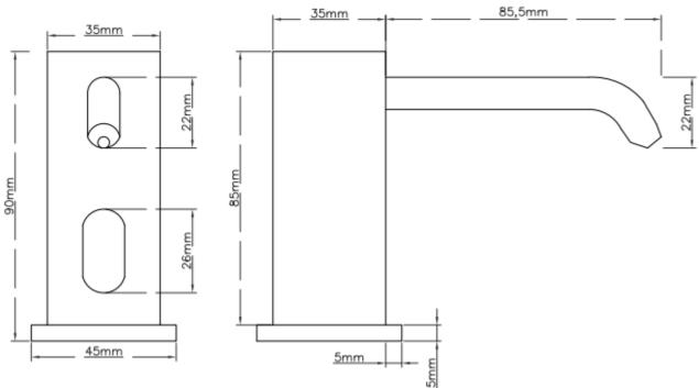
Materials: Constructed from Type UK 304 stainless steel, 0.9mm gauge with exposed surfaces in a polished finish.
