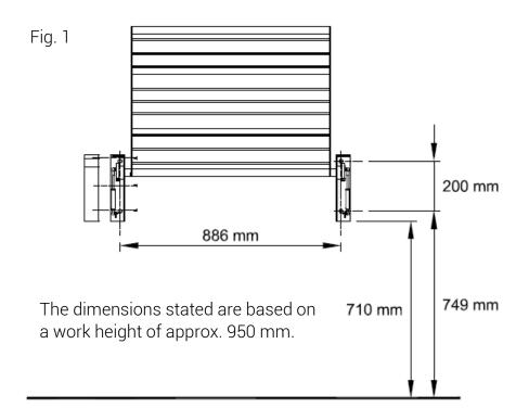
**IMPORTANT:** Be sure to drill the holes for the mountings exactly vertically underneath each other, or the pneumatic shock absorbers inside the mountings may break.
